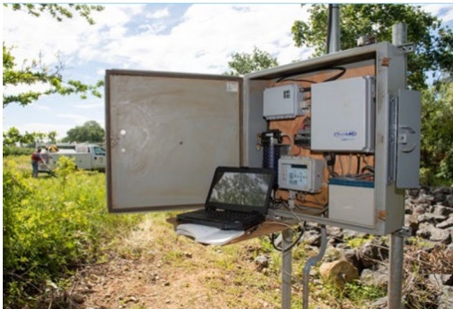
Stream Gage Improvement Program (CalSIP) Technician performing work on a digital stream gage.
